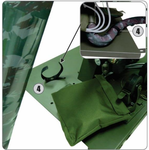
7 - Attach the corrugated hose to the strap (4) attached to the base of chair.
