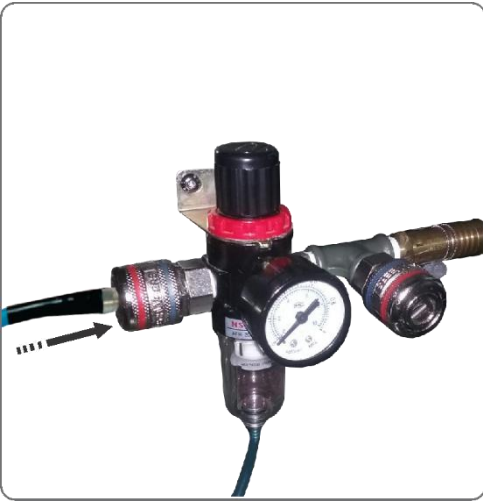
2 - Disconnect the compressed air supply hose from the equipment.
