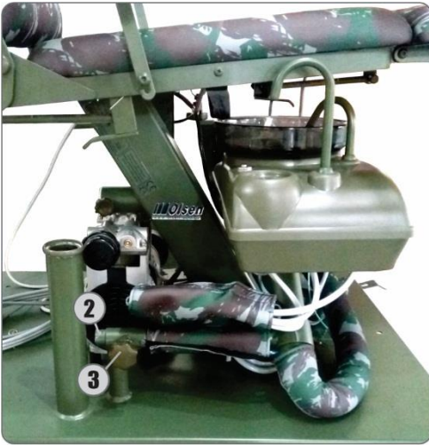
6 - Pass the water unit under the seat and attach it to the holder (2) on the right side of the unit; lock the handle (3).
