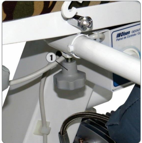
5 - To remove the water unit, Release the water unit locking handle (1), store it with the hoses and instruments in the package; If the equipmente has a curing light and/or ultrasonic scaler, disconnect it and store it in the stainless steel tray and instrument package.
